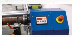
Automatic tensioning with 4 presets, large digital display, and 0.01 mm cutting accuracy.
